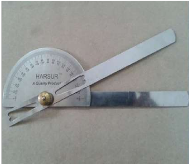
Fig 2: Goniometer used to measure Q angle
